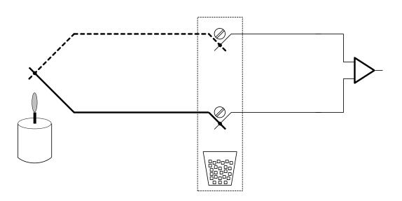
From Table 1, we see that the selection of a specific T/C type will be guided by the useful measurement range of the sensor, its sensitivity, its material, and its operating environment. Sensor cost may also play a role in this decision as certain types are more expensive than others—for example, the platinum based sensor types are generally more expensive by virtue of their platinum content.
